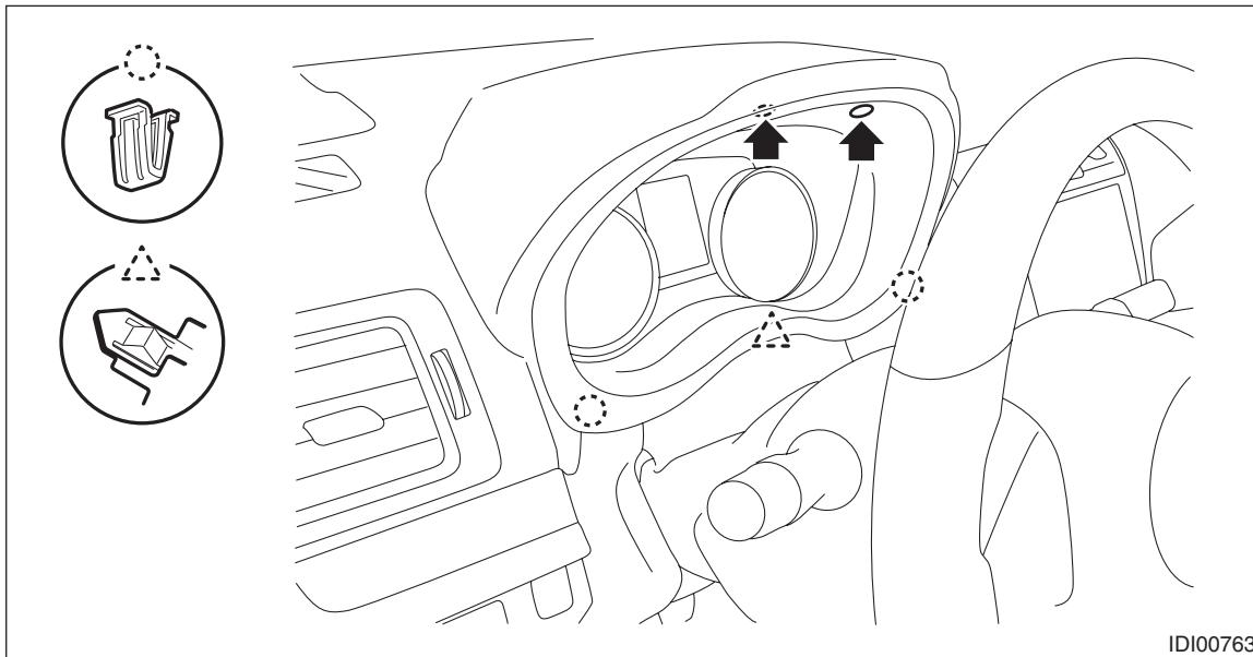
4) Remove the combination meter assembly.
